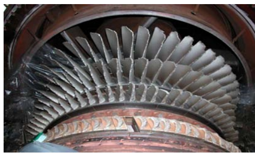
(a) Broken rotor from the first to the fourth row blades
